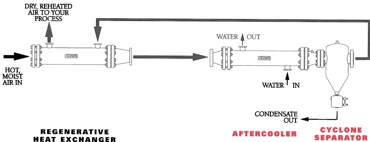
**FIGURE 5 THE ECONOMAT SYSTEM, USING TWO COOLING SOURCES**
