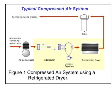
Cooling compressed air is an essential method to condense moisture that is present in the stream. However, it robs the energy or volume from the compressor system. While the amount can vary, it is not unusual to lose thirty percent of the energy available from the total compressed air system.
