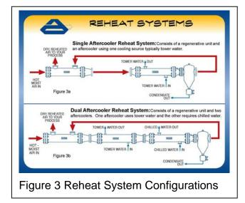
The Economat Reheat system configuration can vary as seen in Figure 3. Figure 3a shows a Reheat System that uses one aftercooler. The aftercooler cooling medium can be cooling tower water, chilled water, river water, lake water, or city water.
