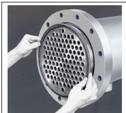
Figure 16. First packing ring installation.
