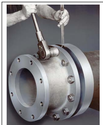
Figure 20. Tightening of the packing gland.
