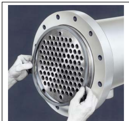
Figure 18. Second packing ring installation.
