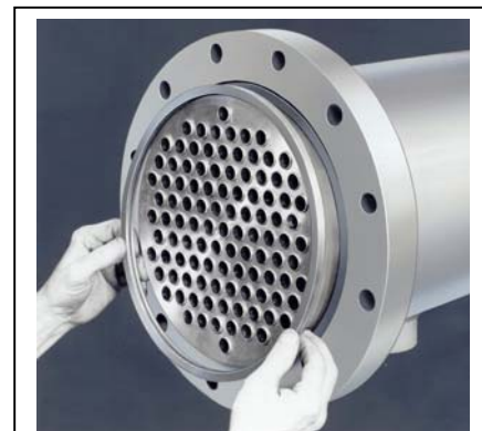
Figure 17. Vent ring installation.
